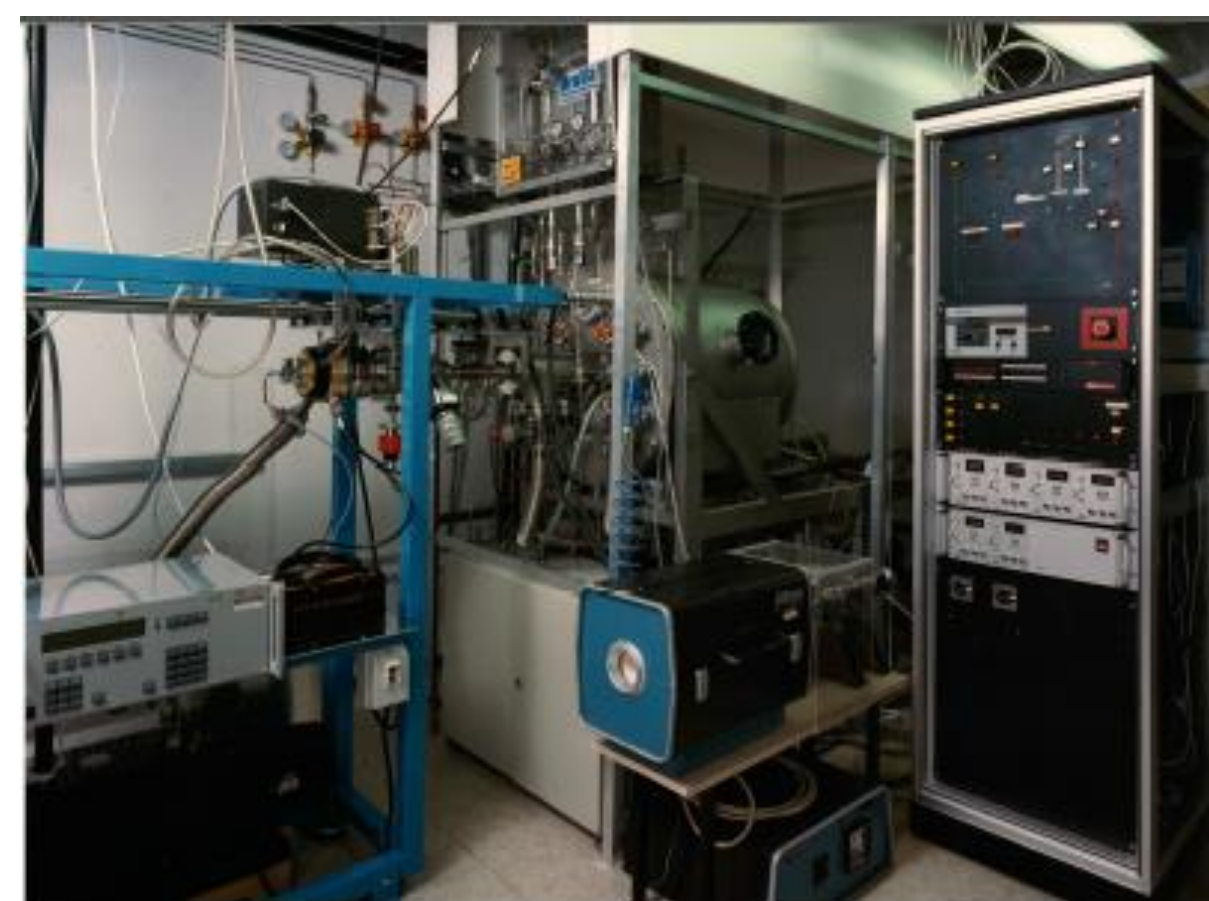
ALE reactor built for III-V growth at the Semiconductor Laboratory, VTT Technical Research Centre of Finland, basement in Otakaari 7B, Otaniemi, Espoo. III-V research was conducted at VTT by Ilkka Suni, Jouni Ahopelto and Hannu Kattelus. Precursors were gallium and indium chlorides and arsine. The reactor was initially tested by depositing GaN and AlN. Photo is 1987 and was provided to the exhibition by Prof. Jouni Ahopelto.
