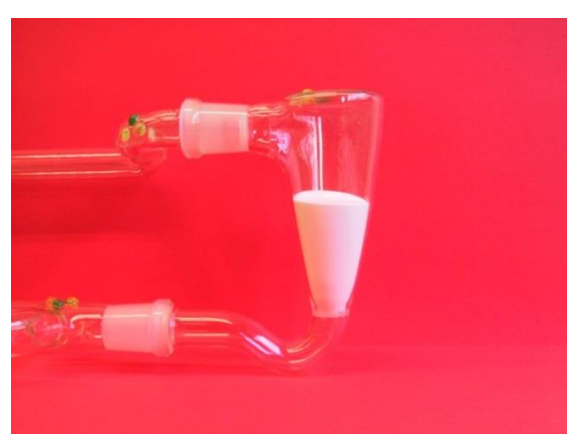
Fluidized bed reactor insert for an F-120 reactor, for creating ALD coatings on particles. The reactor has been used for catalysis ALD research at the University of Joensuu. Photo provided by Prof. Tapani Pakkanen.
