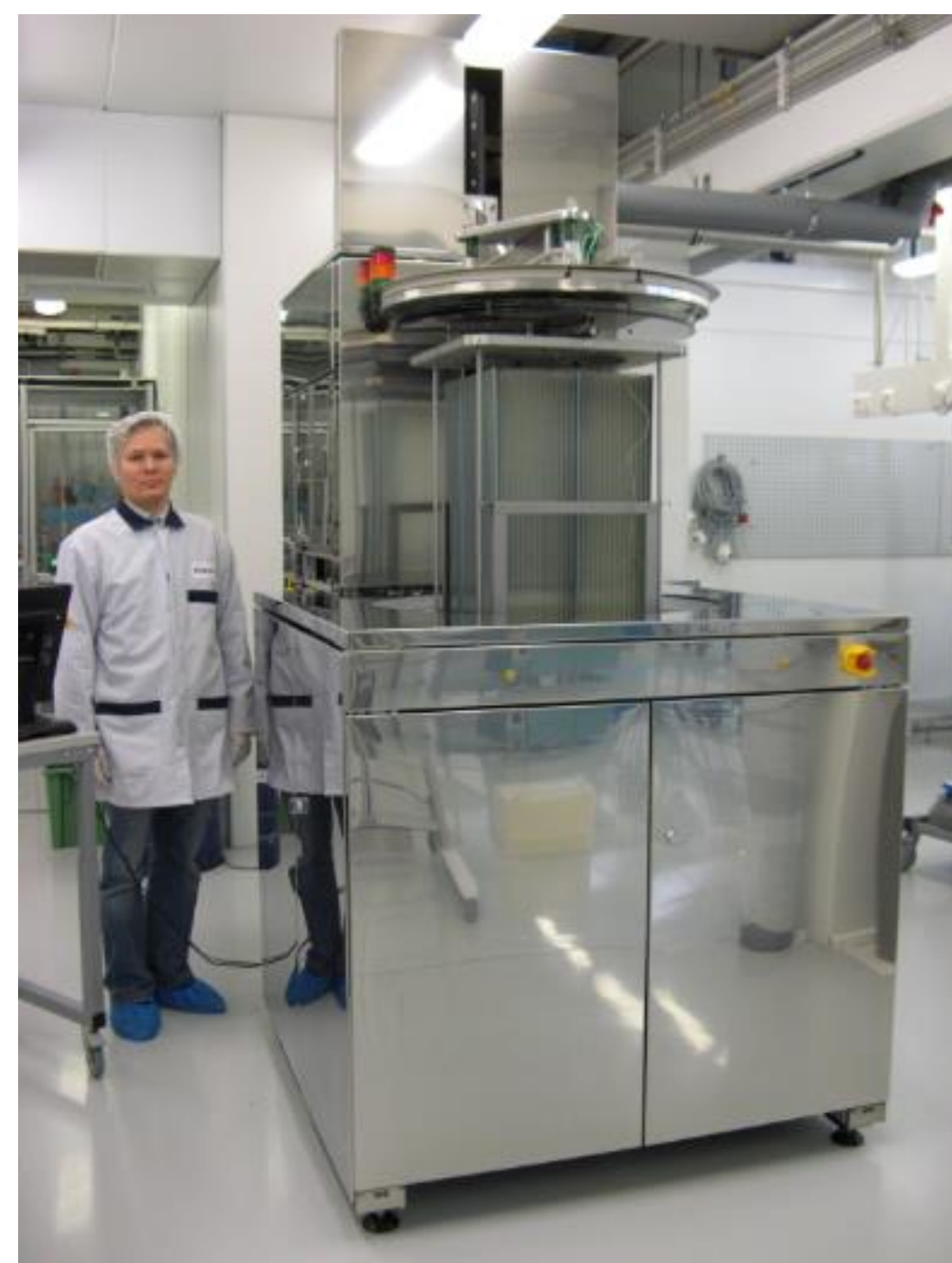
PICOSUN™ P-1000 ultra-large scale batch ALD reactor prototype in 2013, with Dr. Marko Pudas. Photo provided to the exhibition by Dr. Minna Toivola.
