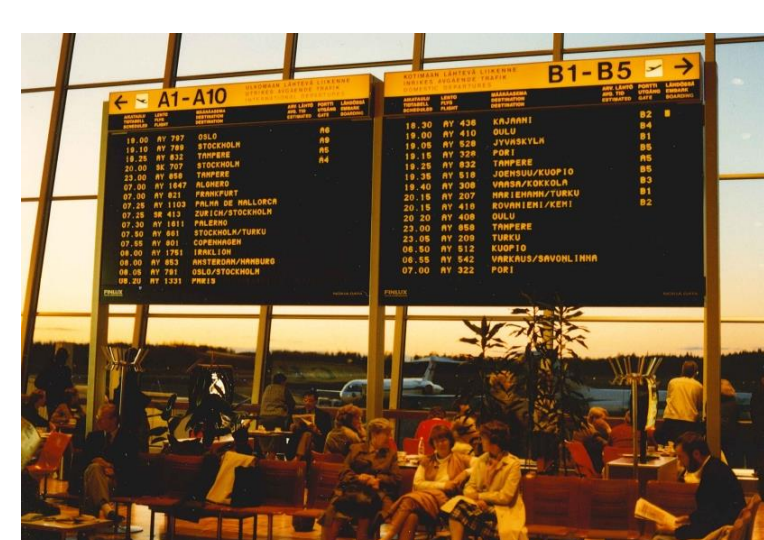
Flight display modules with ALD (ALE) TFEL character units at Helsinki-Vantaa airport, 1983. Photo courtesy of Beneq Oy.
